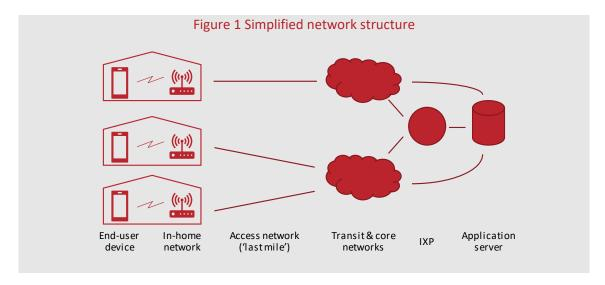
For example, the in-home network and the 'last mile' (the link between a house and the nearest telephone exchange) are both exclusive to that home. Any congestion in these components will be a result of usage in that home, not the result of heavy usage in other households.<sup>2</sup>
